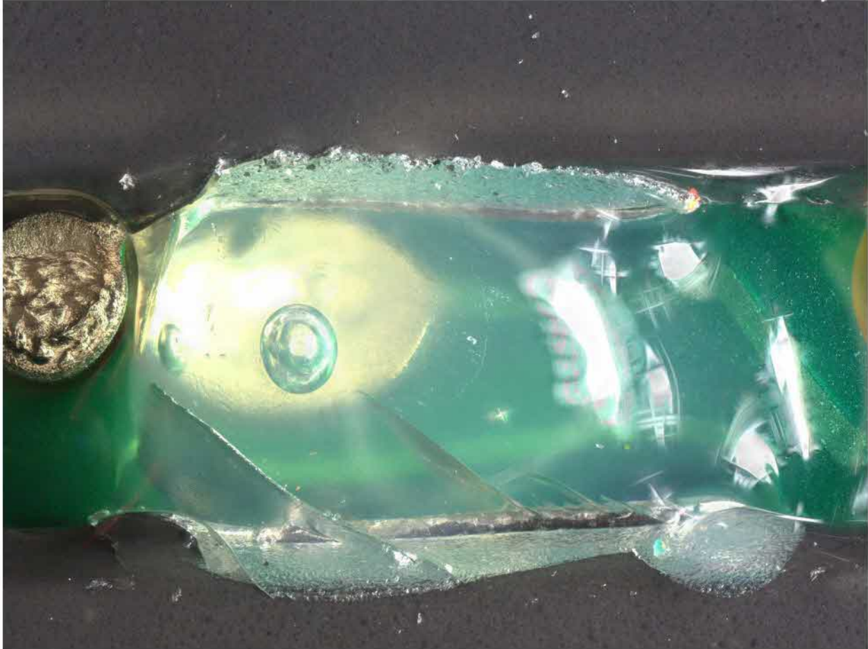
Figure 9. Example of cracks seen in epoxy bond between chips U1 and U2.
